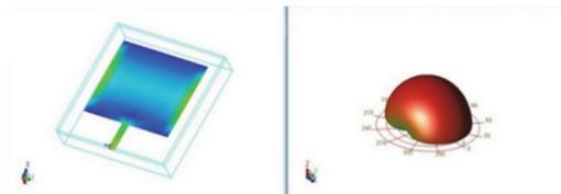
Fig. 5. Patch antenna radiation pattern.
