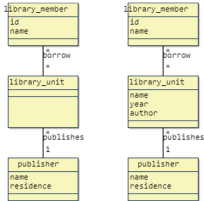
Fig. 7. CDM derived from recorded speech without text modification (left), and after text modification (right).
