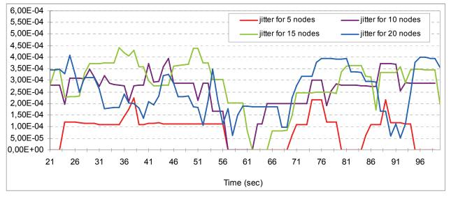
Fig. 5. Comparing jitter for different numbers of mobile nodes.
