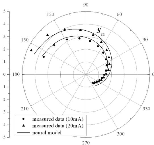
Fig. 6. Scattering parameter  $S_{21}$ .
