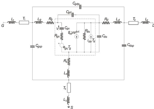
Fig. 1. Equivalent circuit of MESFET / HEMT package including noise sources.
