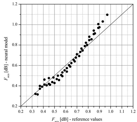
Fig. 5. Minimum noise figure – a scatter plot of neural model output vs. reference values.
