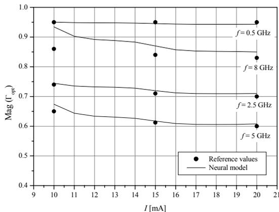
Fig. 8. Magnitude of optimum reflection coefficient vs. bias current.
