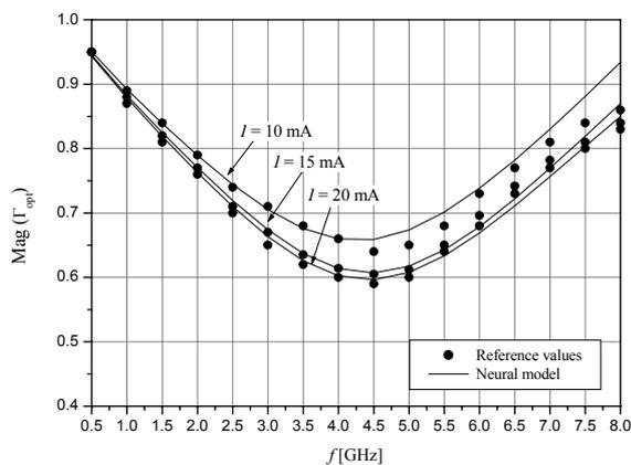
Fig. 7. Magnitude of optimum reflection coefficient vs. frequency.
