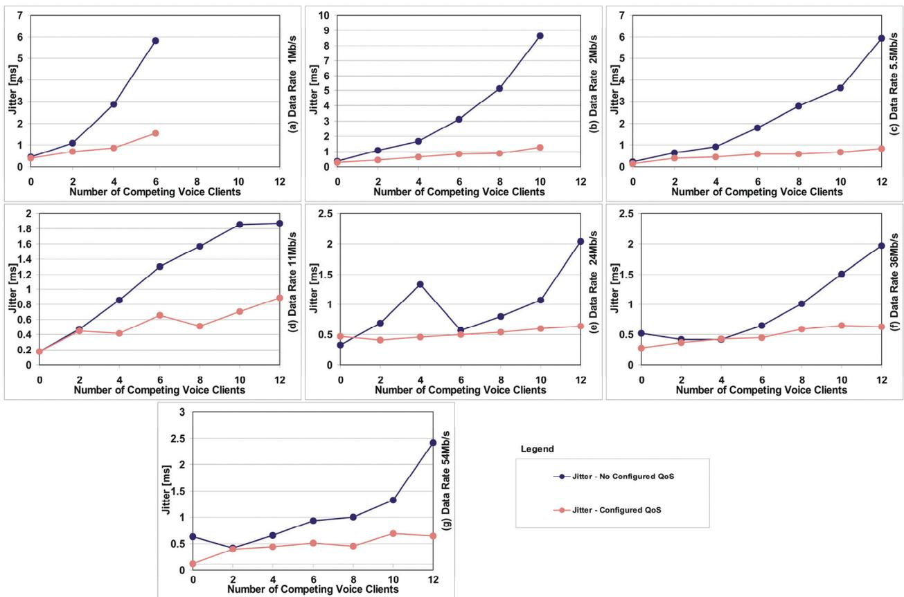
Fig. 7. Mean jitter depending on number of competing voice clients and data rates for measuring topology Case 1.
