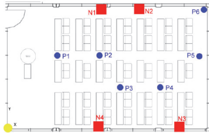
Fig. 5. The layout of the testing room (classroom) with combination of plastic slices and aluminum walls.
