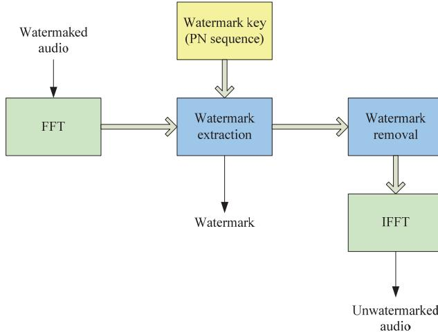
Fig. 4. Extraction and removal scheme.
