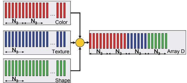
Fig. 3. Merging resulting arrays of image IDs after ranking in group of features.
