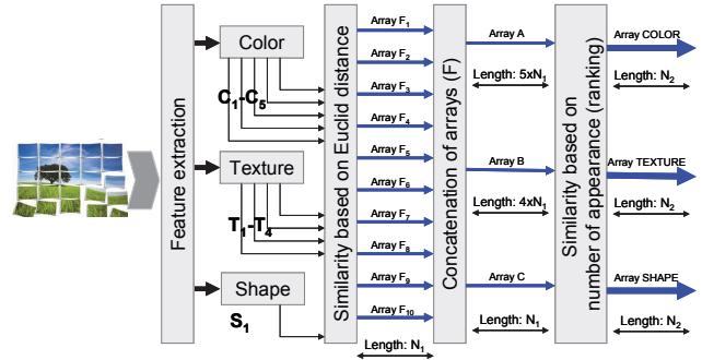
Fig. 2. Initial searching procedure based on individual features and Ranking algorithm.
