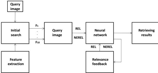
Fig. 1. Functional scheme of the proposed CBIR system based on automated selection of relevant images.
