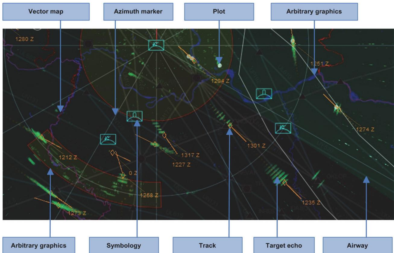
Fig. 4. Elements of the air situation picture as displayed by DRI.
