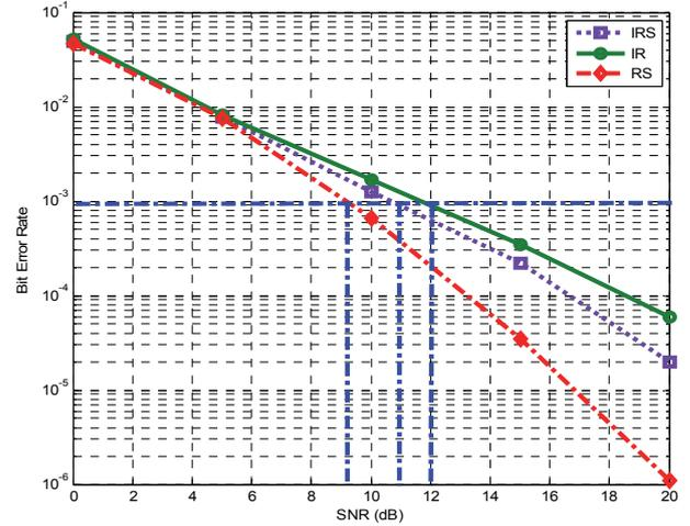
Fig. 2. BER comparison for the 2111 ( $n_{tr}^s = 2$ ,  $n_{rc}^{r_k} = 1$ ,  $n_{tr}^{r_k} = 1$ ,  $n_{rc}^d = 1$ ) scenario,  $\gamma_{th} = 5$  dB and  $M=2$ .
