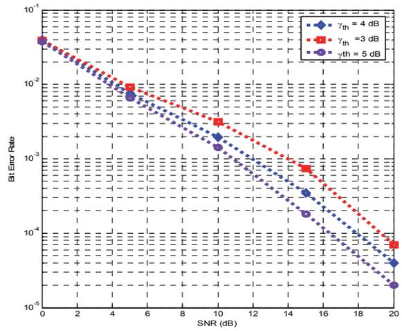
Fig. 3. BER performance of OSTBC-MIMO system with DF incremental relay selection for different values of  $\gamma_{th}$  for the 2111 scenario.
