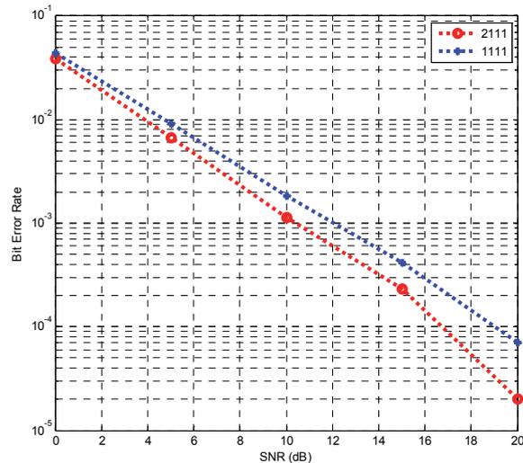
Fig. 4. BER performance of DF incremental selective MIMO relaying and SISO relaying for  $\gamma_{th}=5$  dB,  $M=2$ .
