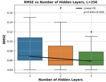
Fig. 9. RMSE values for different numbers of LSTM layers, and for a fixed number of units  $L = 256$ .
