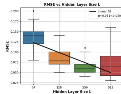
Fig. 8. RMSE values for different numbers of hidden units L in the LSTM block.
