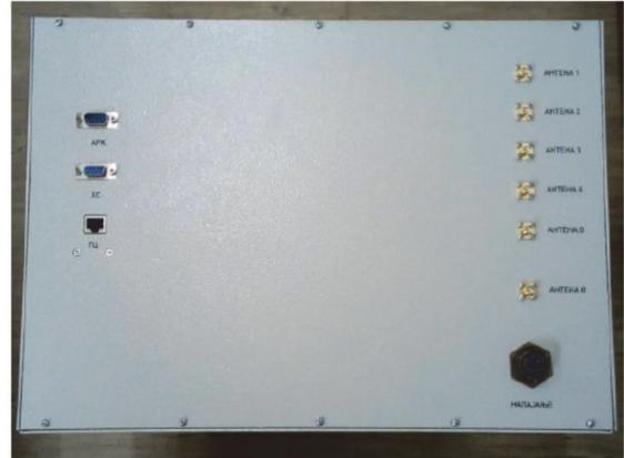
Fig. 7. The rear side of VHF/UHF receiver.
