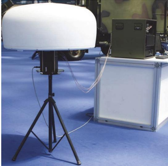
Fig. 1. VHF/UHF direction finding system.
