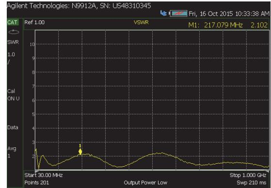
Fig. 10. Voltage Standing Wave Ratio (VSWR) for one of the inputs to ARK3600.
