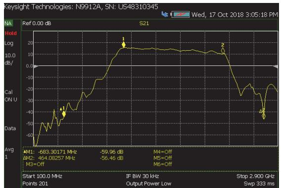
Fig. 12. Filter characteristic as a function of frequency for one of preselector filters at the input of VHF/UHF receiver.
