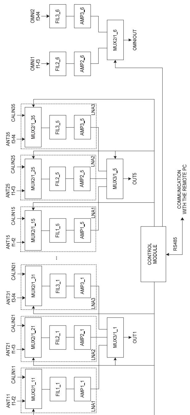
Fig. 2. Block-scheme of antenna multicoupler unit ARK 3600.
