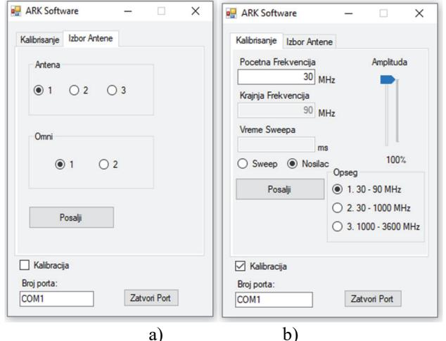
Fig. 5. ARK 3600 network management over communications port: a) antenna selection tab; b) calibration tab
