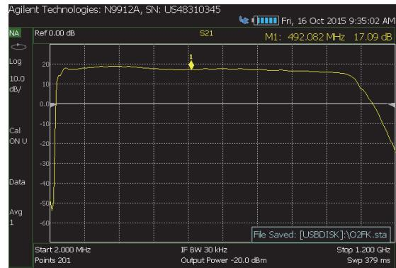
Fig. 11. Filter characteristic as a function of frequency for one of the inputs of ARK 3600.
