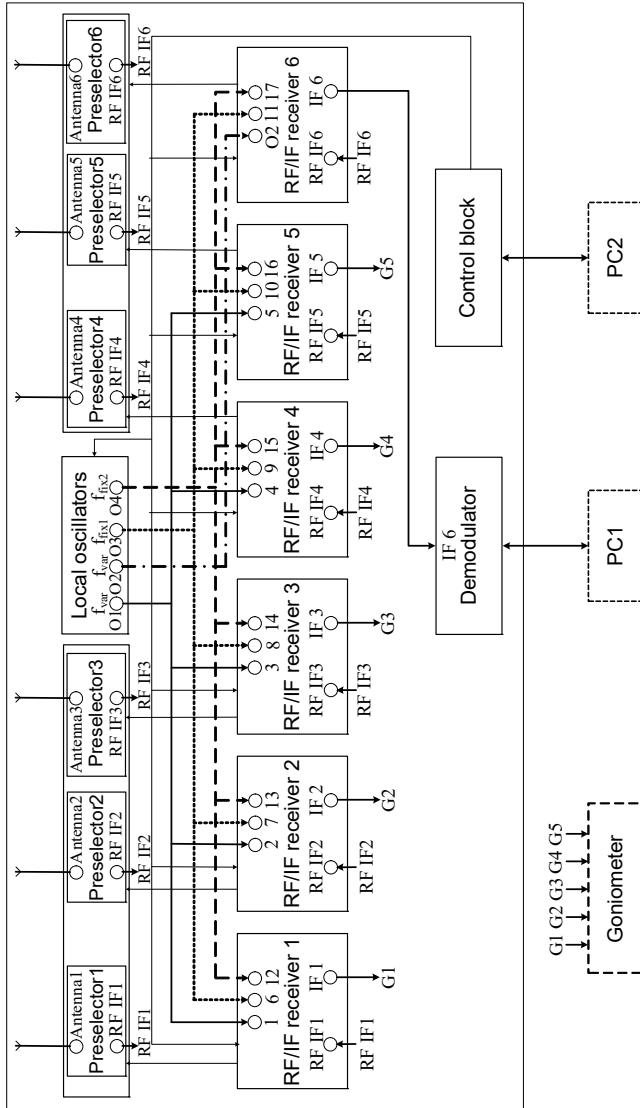
Fig. 6. Block-scheme of the VHF/UHF receiver.
