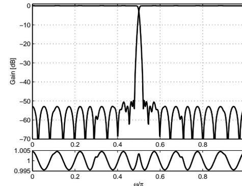
Fig. 8. Frequency responses of low-pass/high-pass filter pair  $[H_{a0}(z), H_{a1}(z)]$ , and verification of nearly perfect power-reconstruction property.
