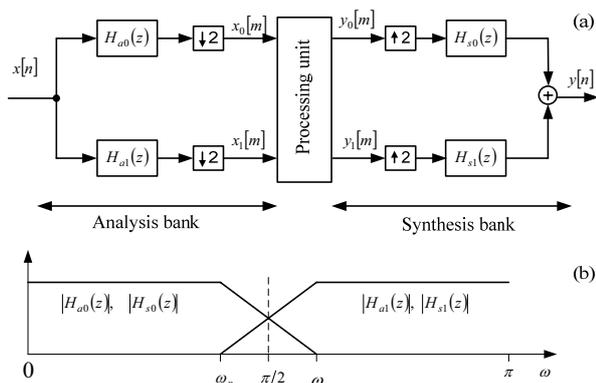
Fig. 1 Two-channel maximally decimated filter bank: (a) Block diagram. (b) Channel division.
