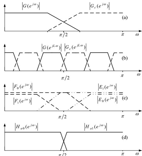
Fig. 2. Generating the analysis filter bank with the aid of FRM approach.
