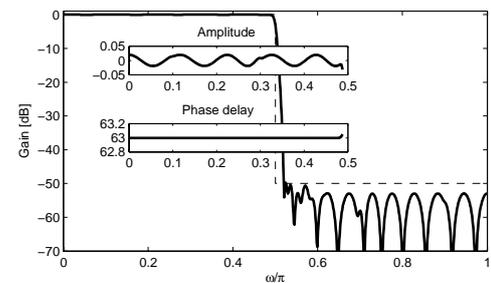
Fig. 7. Frequency responses of low-pass filter  $H_{a0}(z)$ .
