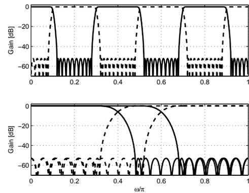
Fig. 6. Frequency responses of: periodic model filter pair; masking filters
