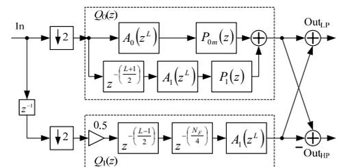
Fig. 4. Efficient realization structure of the analysis bank.
