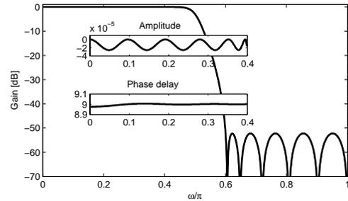
Fig. 5. Frequency response of the low-pass model filter  $G(z)$ .
