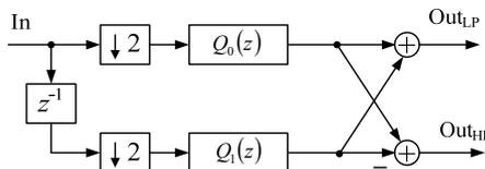
Fig. 3. Polyphase realization of the analysis bank.
