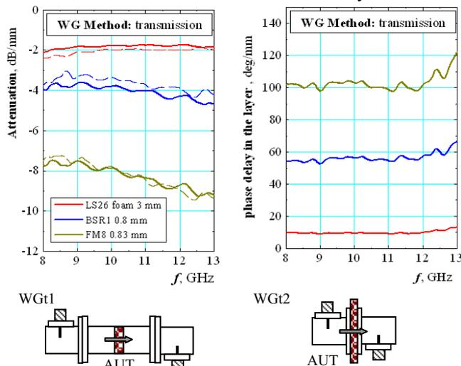
Fig. 3. Measured attenuation and phase delay in three absorbing samples by waveguide transmission-type methods: solid lines (WGt1); dashed lines (WGt2).
