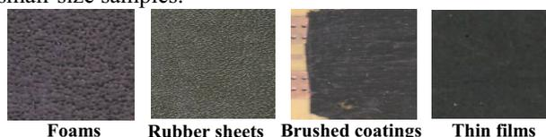
Fig. 1. View of the surfaces of the most popular planar absorbers.
