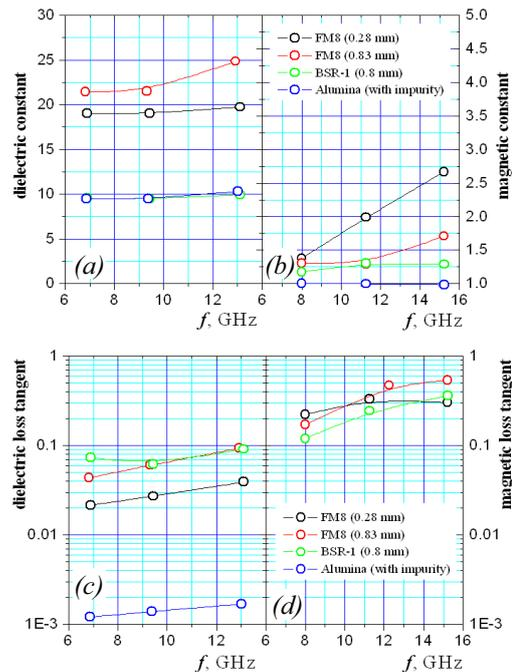
Fig. 10. Results obtained by two-resonator method for dielectric constant (a), magnetic constant (b), dielectric loss tangent (c) and magnetic loss tangent (d).
