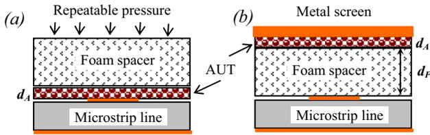
Fig. 6. Fast and accurate planar-line method for determination of the relative absorbing ability of samples with equal thickness  $d_A$ : a) placed directly over 50-Ohms microstrip line (MSL1); b) placed on a metal screen at distance  $d_F$  (MSL2).
