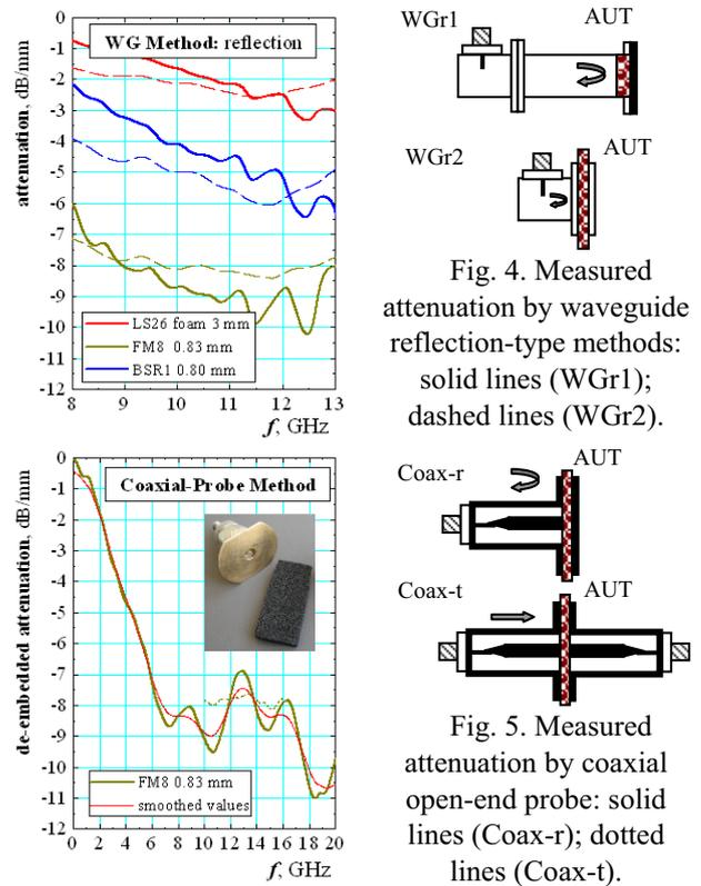
Fig. 4. Measured attenuation by waveguide reflection-type methods: solid lines (WGr1); dashed lines (WGr2).
