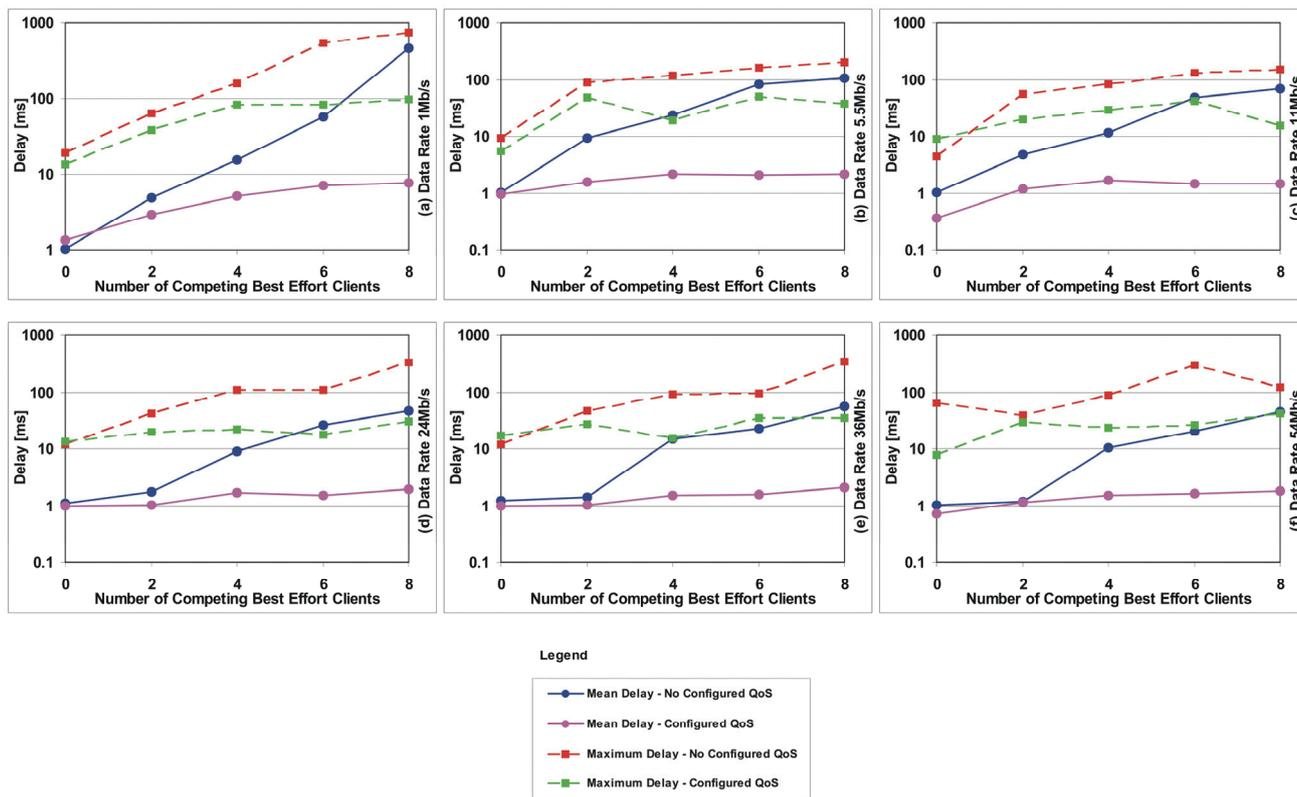
Fig. 4. Mean and maximum delay depending on number of competing best effort clients and data rate for measuring topology Case 1.
