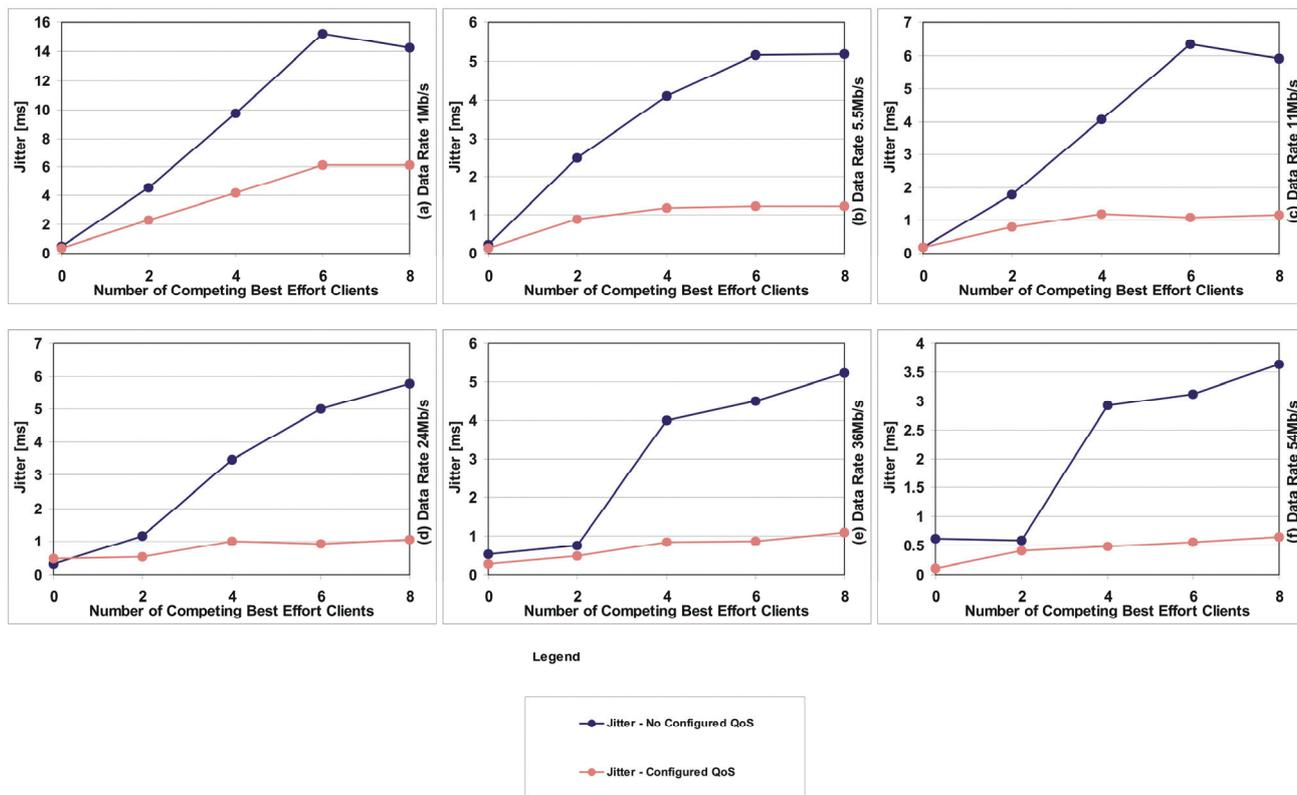
Fig. 5. Mean jitter depending on number of competing best effort clients and data rates for measuring topology Case 1.
