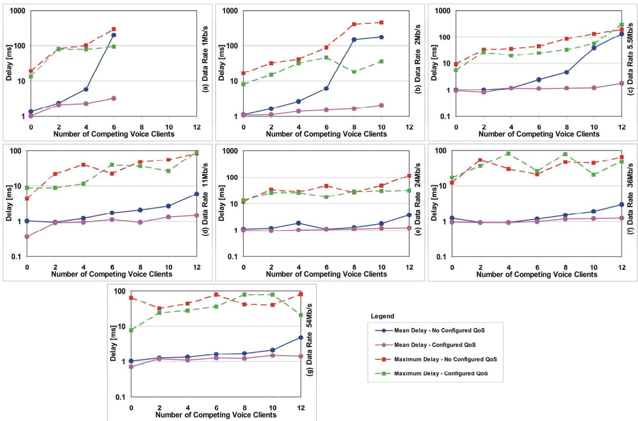
Fig. 6. Mean and maximum delay depending on number of competing voice clients and data rate for measuring topology Case 2.
