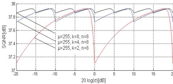
Fig. 3. SQNR for a model with two, four or eight quantizers for the Gaussian source.
