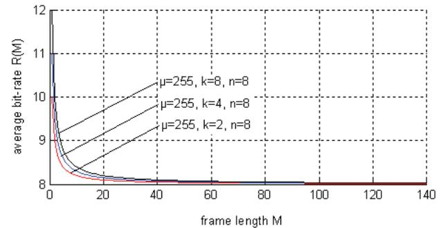
Fig. 5. Average bit-rate for the quantizer with adaptation to average power and speech signal distribution
