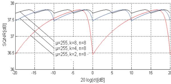
Fig. 2. SQNR for a model with two, four or eight quantizers for the Laplacian source.
