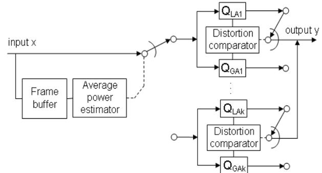
Fig. 4. Switched adaptive scalar quantization with adaptation to average power and speech signal distribution
