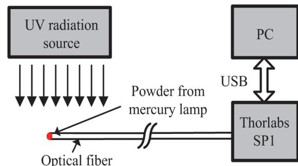
Fig. 3. The block diagram of experimental setup for end-type fiber-optic UV radiation sensor.
