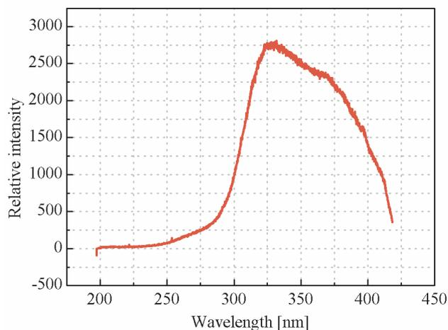
Fig. 6. UV spectrum of solar simulator.
