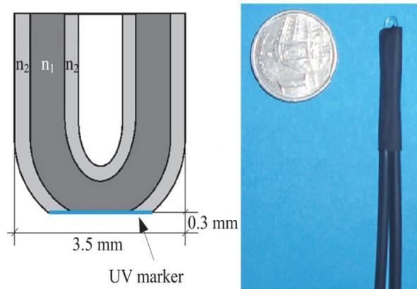
Fig. 2. U-shaped sensor.
