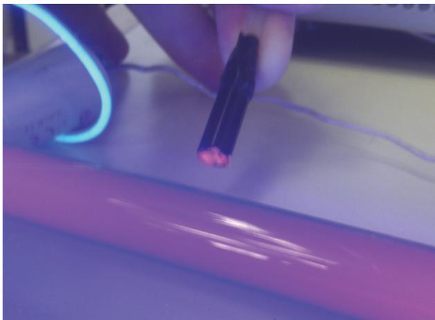
Fig. 4. End-type sensor with powder from mercury lamp.
