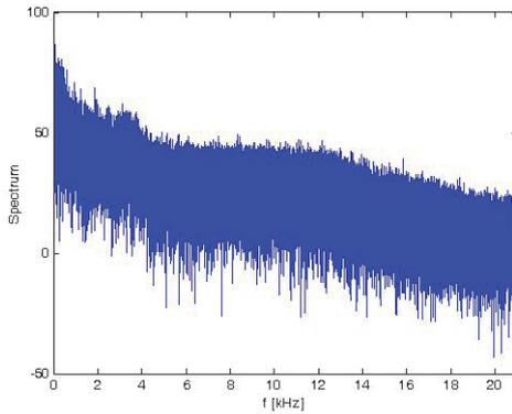
Fig. 6(b). Recovered signal using technique 2 in frequency domain.
