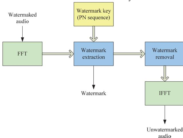
Fig. 4. Extraction and removal scheme.
