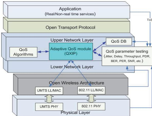
Fig. 1. ME with Adaptive QoS Module.
