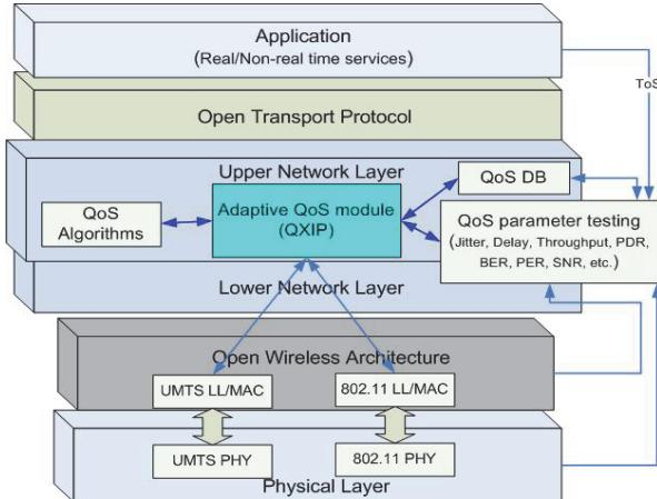
Fig. 1. ME with Adaptive QoS Module.
