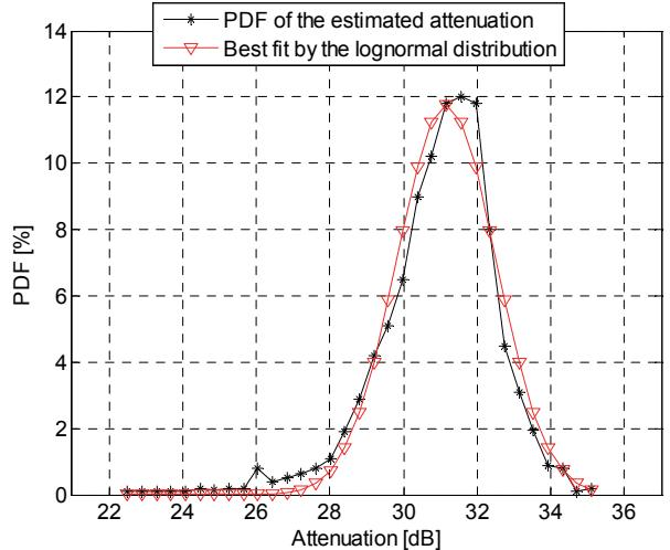
Fig. 7. Histogram of the attenuation and the best fit by lognormal distribution.
