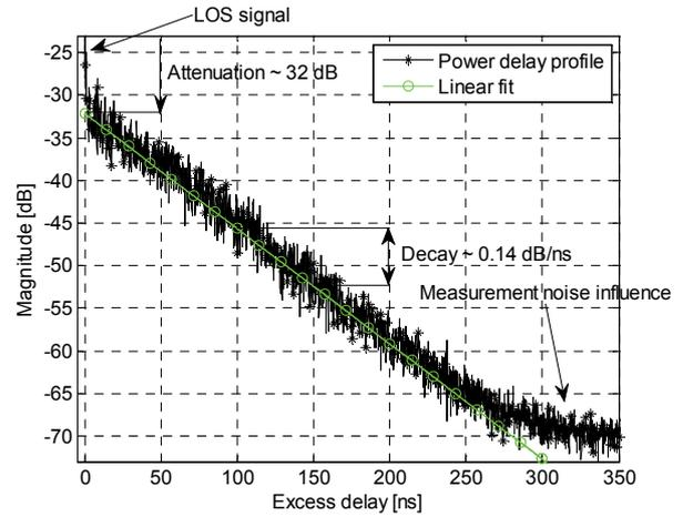
Fig. 6. Signal power as a function of time delay.
