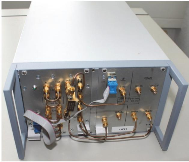
Fig. 4. 1Tx 2Rx baseband module and the up-down converter in an external casing.
