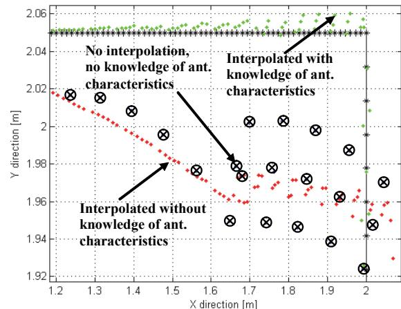
Fig. 10. Location estimation of a moving Tx antenna.
