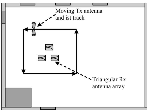
Fig. 9. Ground-plan of the measurement scenario.
