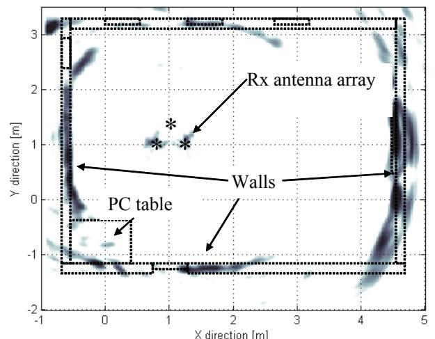
Fig. 11. Imaging of the propagation environment.
