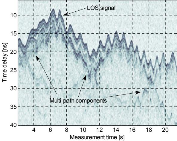
Fig. 5. Example of CIRFs measured in real-time.
