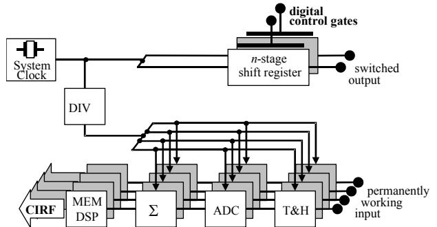
Fig. 2. Example of a parallel 2Tx 4Rx MIMO UWB channel sounder.
