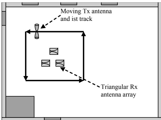
Fig. 9. Ground-plan of the measurement scenario.
