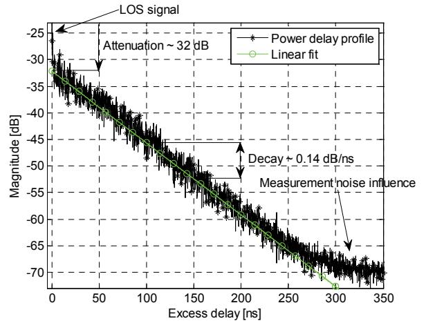
Fig. 6. Signal power as a function of time delay.
