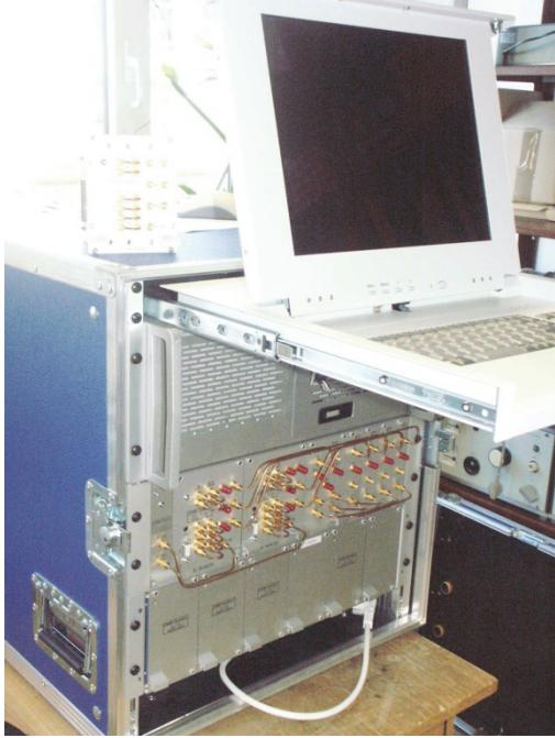
Fig. 3. Construction of the real-time 2Tx 4Rx MIMO UWB channel sounder.
