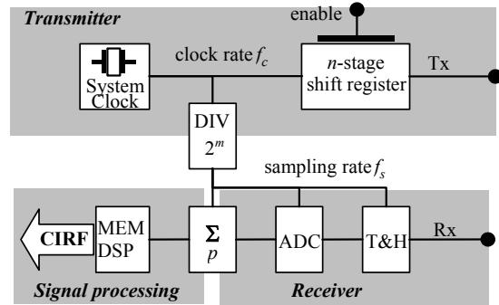
Fig. 1. Basic architecture of the baseband UWB channel sounder.
