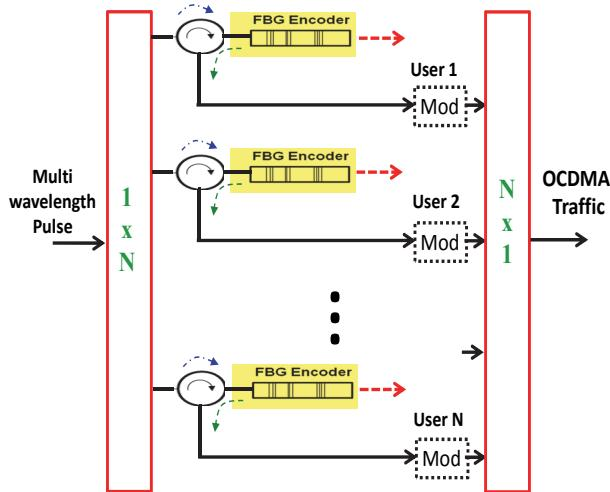
Fig. 5. Architecture of a multiuser OCDMA signal generation. The input multiwavelength pulse is splitted  $N$  times and distributed to each of the FBG based OCDMA transmitters representing up to  $N$  simultaneous users. Mod-Modulator.
