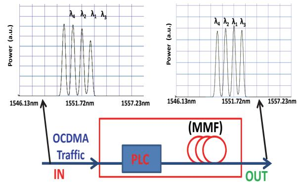
Fig. 9. Illustrating technique used to optically process in-situ an FGB based 2D-WH/TS code. The optical spectrum of the input un-equalized code and the resulting output equalized code is shown.
