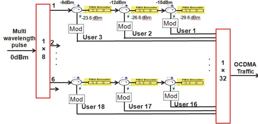
Fig. 7. Modified architecture of the multiuser FBG based OCDMA signal generation. The encoders have been cascaded to enable the reuse of unreflected multiwavelength optical. The input optical splitter has also been replaced with a cheaper alternative. Mod-Modulator.
