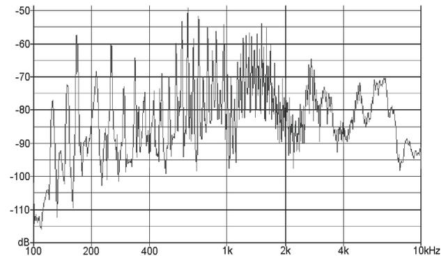
Fig. 12. Vibration spectrum recorded on a violin bow while playing the tone with a frequency of 41 Hz.
