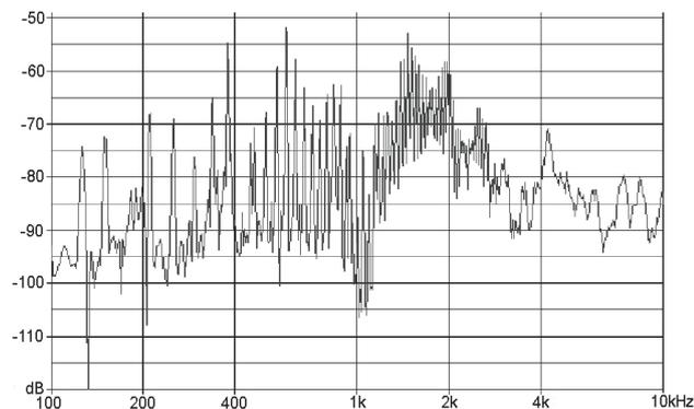
Fig. 11. Vibration spectrum recorded on the French bow while playing the tone with a frequency of 41 Hz.
