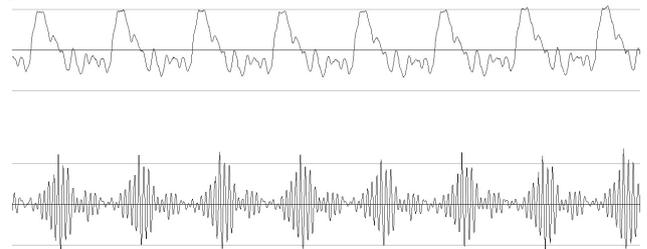
Fig. 4. Sound (above) and vibrations on a bow (below).
