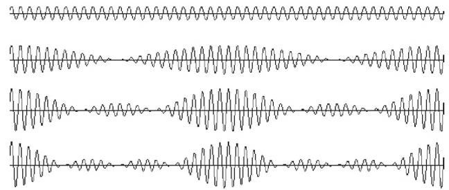
Fig. 7. Graphics obtained by successive summing of sinusoidal signals (from top to bottom: 1025 Hz + 1066 Hz + 1107 Hz + 1148 Hz).
