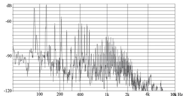
Fig. 5. Double bass sound spectrum recorded while playing tone with a frequency of 41 Hz.
