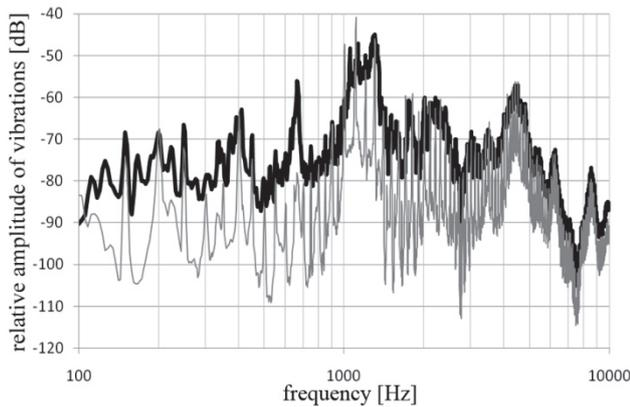
Fig. 6. Vibration spectrum recorded on the bow:
