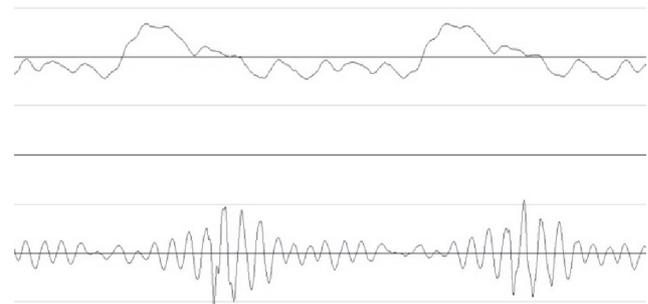
Fig. 8. Sound (above) and vibration (below) - a form of time when playing the tone D (73 Hz).
