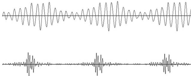
Fig. 9. Components of bow vibration while playing the tone G (98 Hz) - up: 800-2350 Hz, bottom: 2350-7300 Hz.
