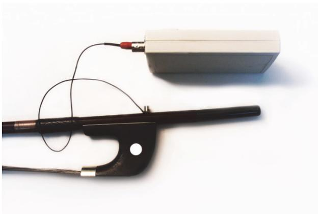
Fig. 3. A vibration sensor installed on a bow stick.
