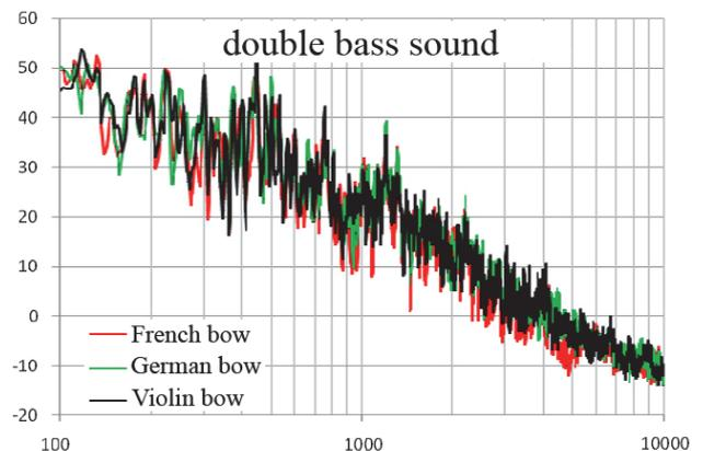
Fig. 13. Comparative review of the double bass sound spectrum for all three types of bows while playing a tone with a frequency of 41 Hz.
