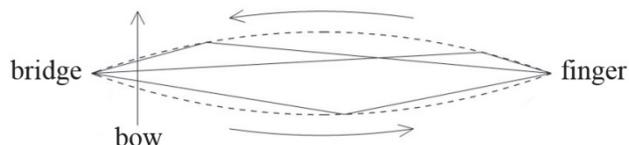
Fig. 1. Bow string interaction causing Helmholtz peak motion.
