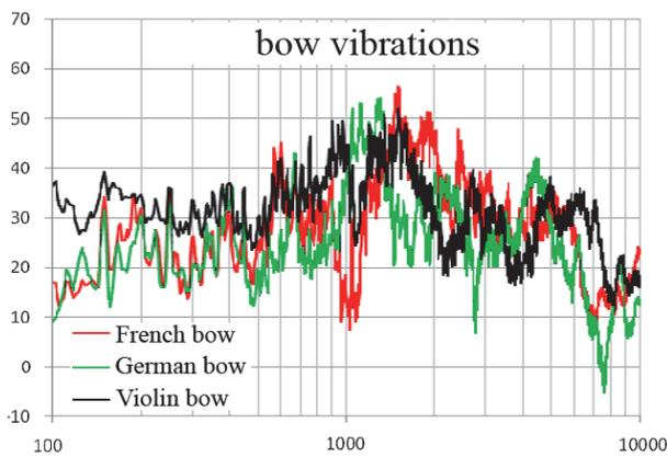
Fig. 14. Comparative review of the bow vibration spectrum for all three types of bows while playing a tone with a frequency of 41 Hz.
