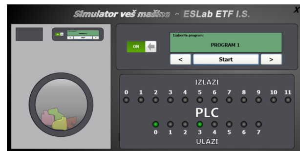
Fig. 6. User interface for washing machine simulator (everything is animated except for door opening).
