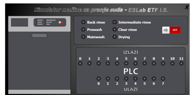
Fig. 7. User interface for dishwasher simulator (everything is animated except for door opening).
