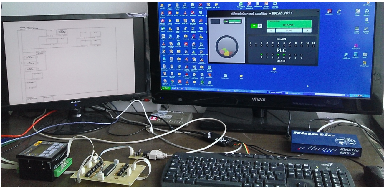
Fig. 9. The complete development environment for monitoring, data acquisition and simulation of PLC controlled applications.
