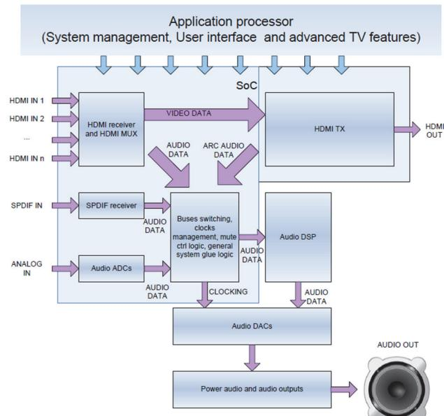
Fig. 2. Block diagram of the sound bar system.
