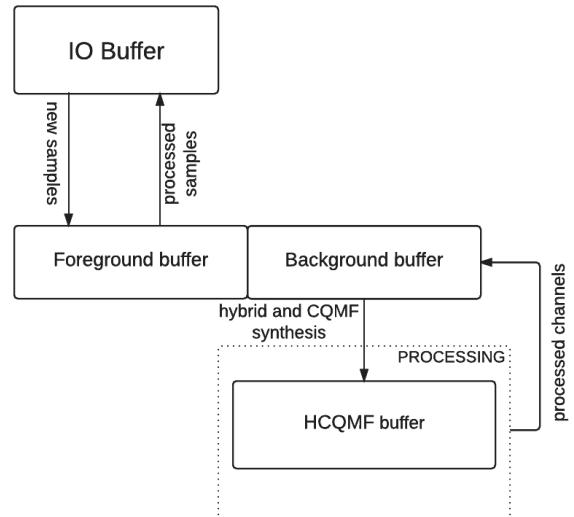
Fig. 6. Block diagram of the implementation.
