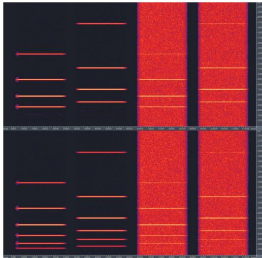
Fig. 8. Spectral view of the Left Surround channel before and after surround virtualization.
