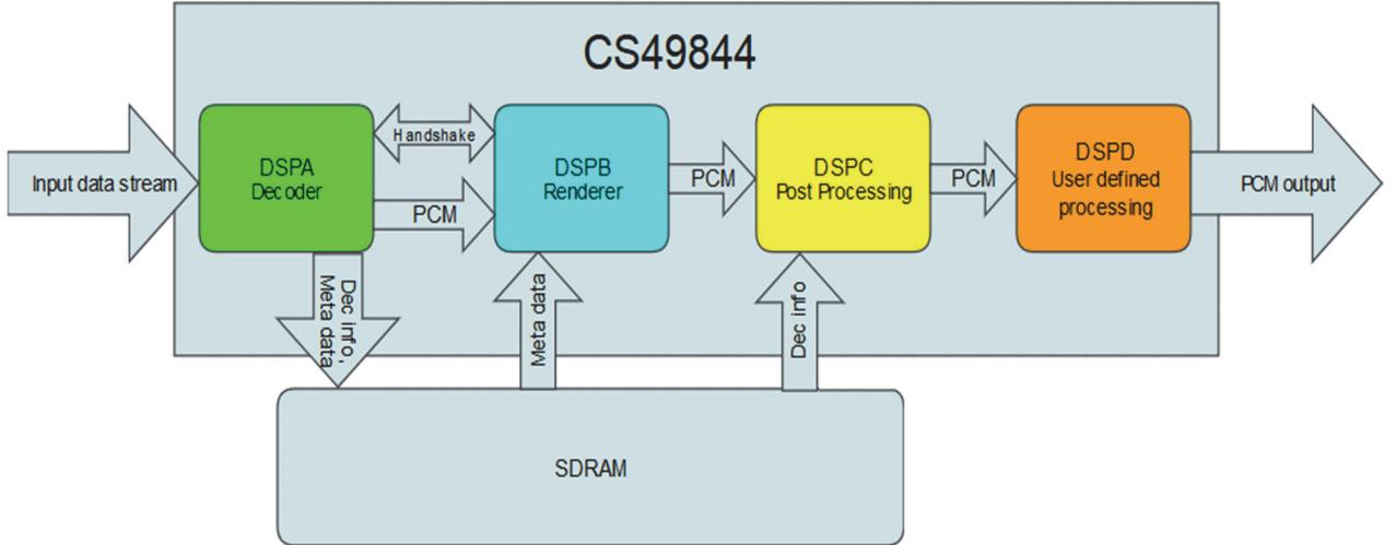
Fig. 4. Allocation of modules in the sound bar system.
