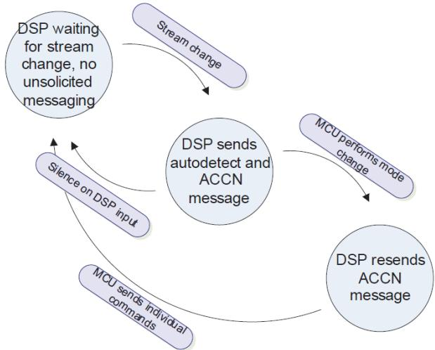
Fig. 3. DSP to Microcontroller Messaging Diagram.
